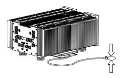
Remove sliding-sheet and shock absorbing feets.
